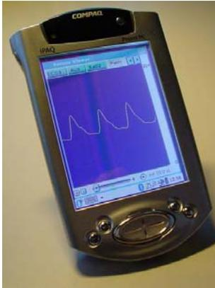
Figure 3 : MBU display – Plethysmogram
