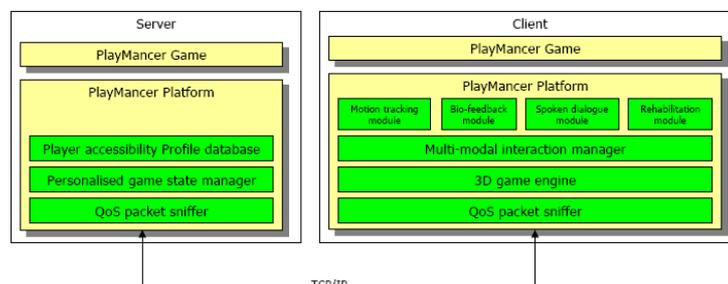
Fig. 1. Deployment of PlayMancer components over the network
