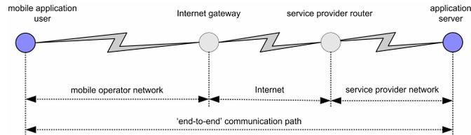
**Figure 1. An 'end-to-end' communication path for a mobile service delivery**
