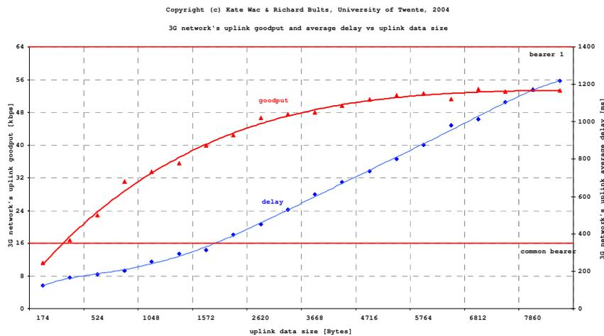
**Figure 3** Performance characteristics of 3G communication network
