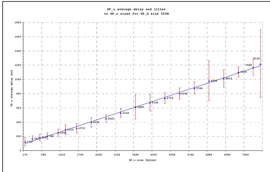
**Figure 8:** Delay and jitter (scale 0 to 1800 ms) for different packet sizes (from 174 to 8022 bytes)
