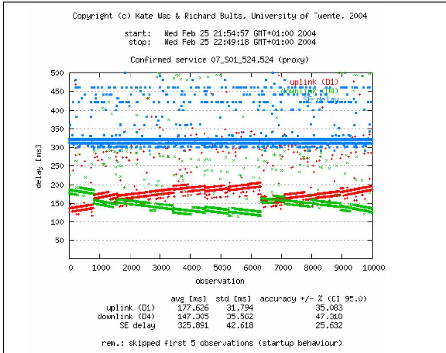
Figure 9: Clock drift influence on the measured delay over a period of 1 hour (uplink, downlink and total delay)
